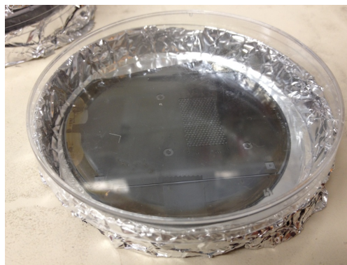
Figure 10.2: Manufacturing the reservoir: Wafer with photoresist features in a petri dish lined with aluminum foil
