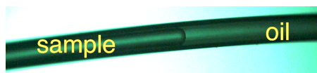
Figure 10.8: Sample in storage layer inlet tubing without trapped air: There must not be air bubbles between both liquid phases for proper loading
