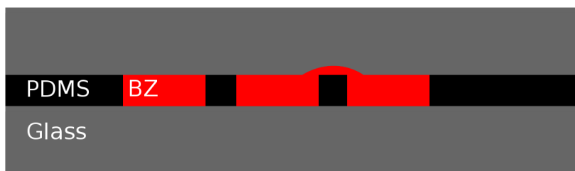
Figure 16: The in-phase oscillations seen in figure 15 were likely caused by a "short circuit" in which ineffective sealing allowed a thin layer of BZ to be between the PDMS and the glass to excitatorily couple neighboring oscillators.
