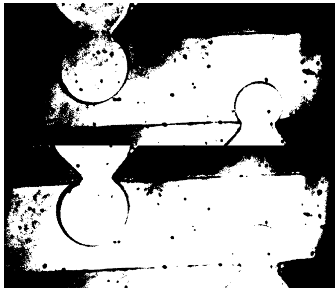
Figure 39: When the drop is lit too harshly, the image processing algorithm will not be able to find any good lower bound threshold value that can capture the entire drop border. The lighting should be uniform throughout the image.
