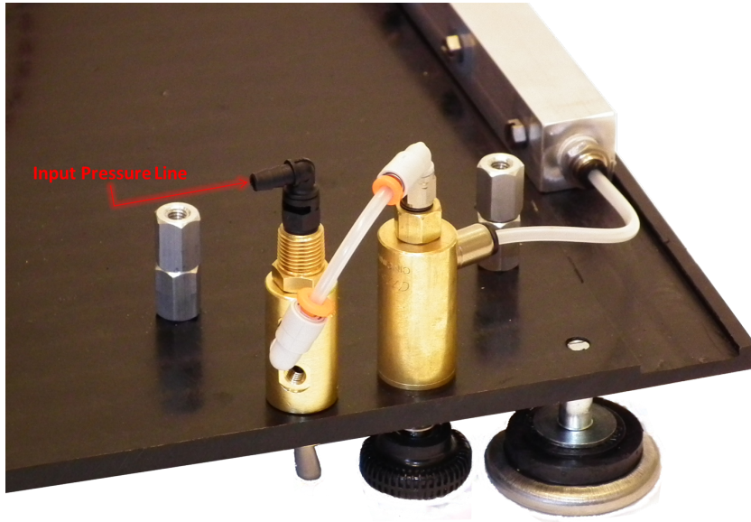
Figure 29: The system shutoff switch connected to the system pressure regulator and distribution manifold. The location for attaching the input pressure line is labeled.
